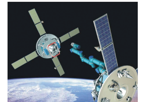
Germany's ROKVISS robot (below) got a workout this year on the space station. A follow-on version (right) might someday service satellites.
